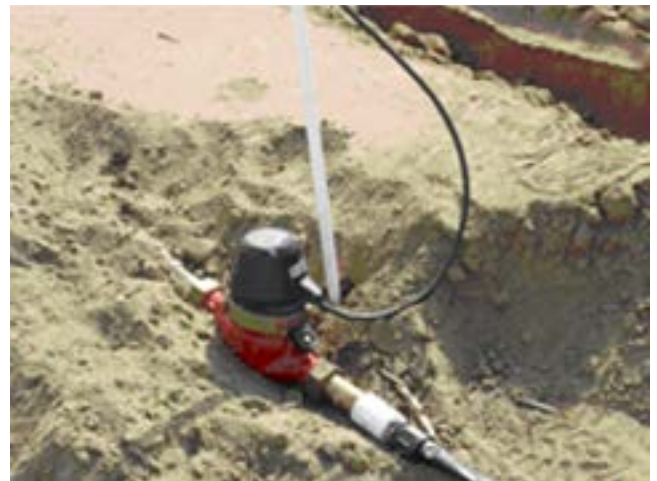
Figure 7–49 Single jet flowmeter inserted into a lateral dripperline and connected to a RF transmitter
