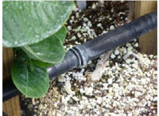
Figure 7-55 Schematic of an early (1967-70) in-line pressure laminar flow emitter (courtesy Netafim USA)
