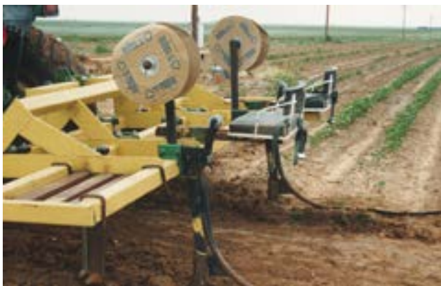
Figure 7-53 Installation of SDI drip tape on a corn field in Texas
