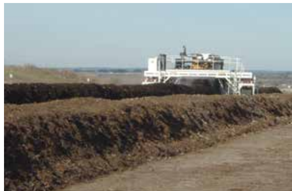
Figure 13.3. Turning a compost pile at a commercial facility. Photo by Alison Jack.
