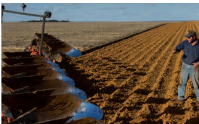
**Plate 6.3** Mouldboard plough in operation for the treatment of non-wetting soil.
