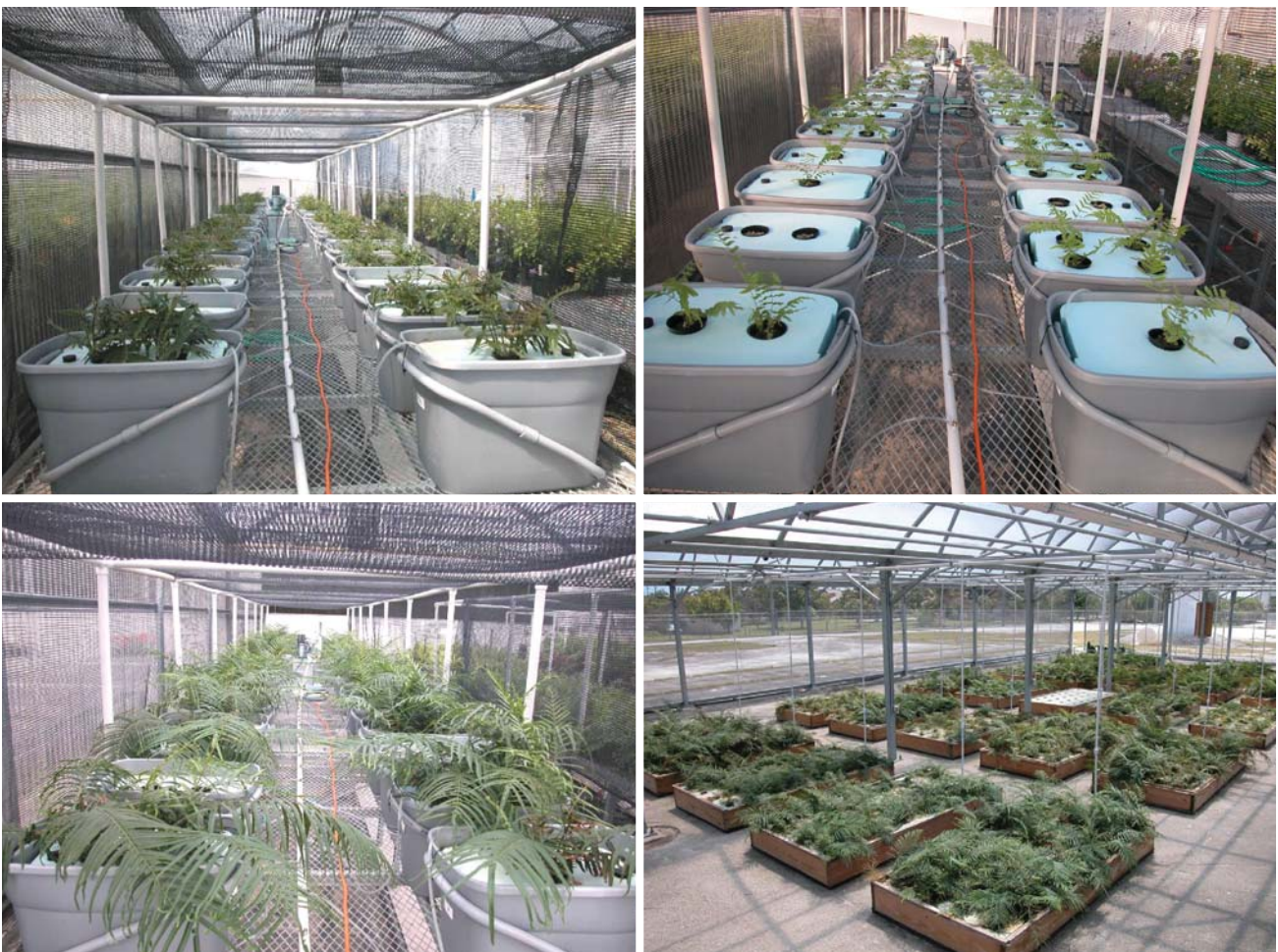
Figure 23. Pilot scale setup using Pteris vittata for removal of As from contaminated water. Courtesy Prof L.Q. Ma. Univ. Florida, USA
