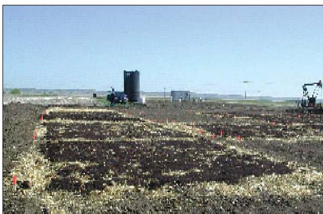
Figure 50. Different stages of bioremediation of oil sludge. Source: Dr. McIntyre T., Environment Canada
