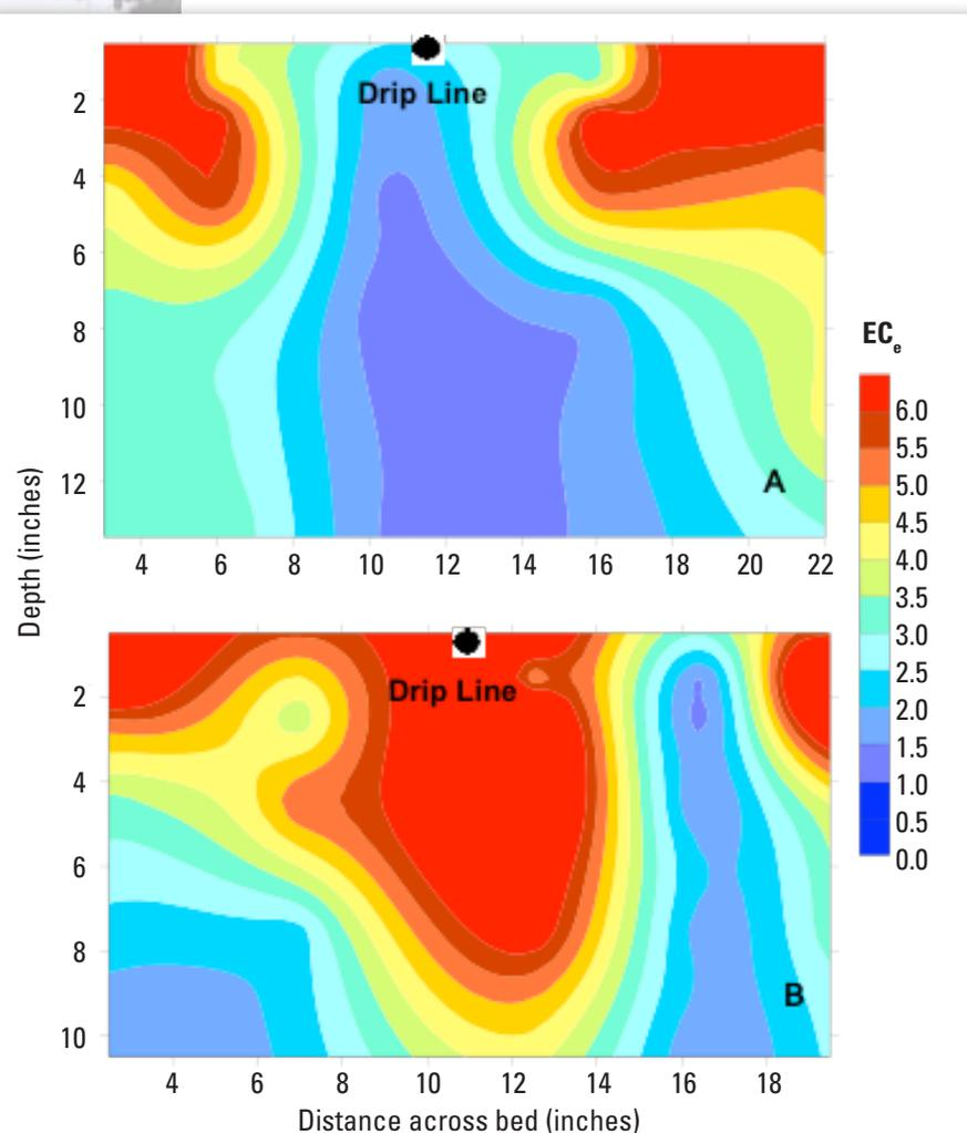
**Figure 6.** Salinity distribution (EC<sub>e</sub>) for (A) leaching around the drip line and (B) no leaching around the drip line. Units of the scale are dS/m.
