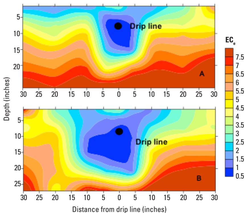
**Figure 7.** Soil salinity ( $EC_e$ ) patterns around a drip line for (A) 12 inches of applied water, and (B) 19 inches of applied water. The low-salt zone around the drip line is larger for the higher amount of applied water. The high levels of soil salinity below the low-salt zones are due to the upward flow of shallow saline groundwater.
