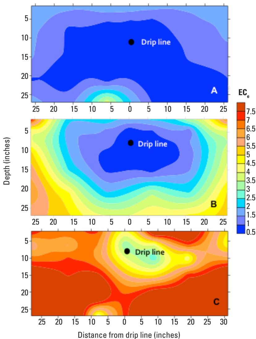
**Figure 5.** Salinity distribution ( $EC_e$ ) n under saline, shallow groundwater conditions for (A) a water table depth of 6 feet and irrigation water with an  $EC$  of 0.3 dS/m, (B) a water table depth of about 3 feet and irrigation water with an  $EC$  of 0.3 dS/m, and (C) a water table depth of about 3 feet and irrigation water with an  $EC$  of 1.1 dS/m. Units of the scale are  $EC_e$  in dS/m.
