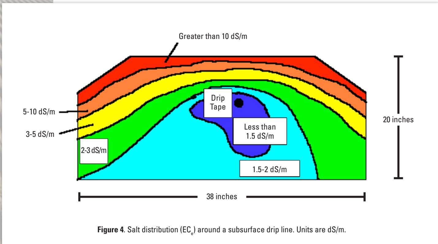
**Figure 4.** Salt distribution (EC<sub>e</sub>) around a subsurface drip line. Units are dS/m.
