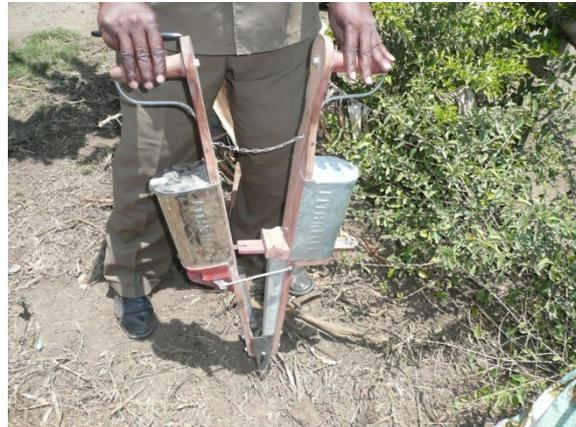
**Figure 7.7 (a). Sketch of a hand-jab planter with seed and fertilizer hoppers**      **(b) A hand-jab planter with seed and fertilizer hoppers** (*photo by Bancy Mati*)
