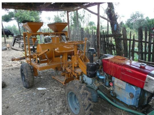
**Figure 7.9 Small 4-wheeled tractor with planter** (photo by Bancy Mati)
