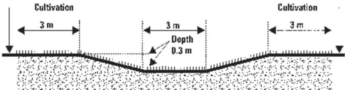
Figure 10-2: Cross-section of a typical grassed waterway<sup>37</sup>
