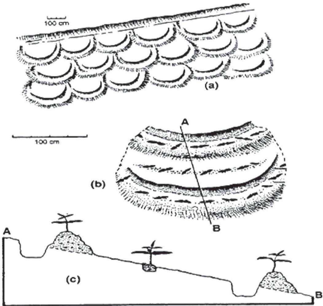
Figure 6-2: Cross sectional views of Katumani pits in plan (a and b) and cross sectional views<sup>24</sup>
