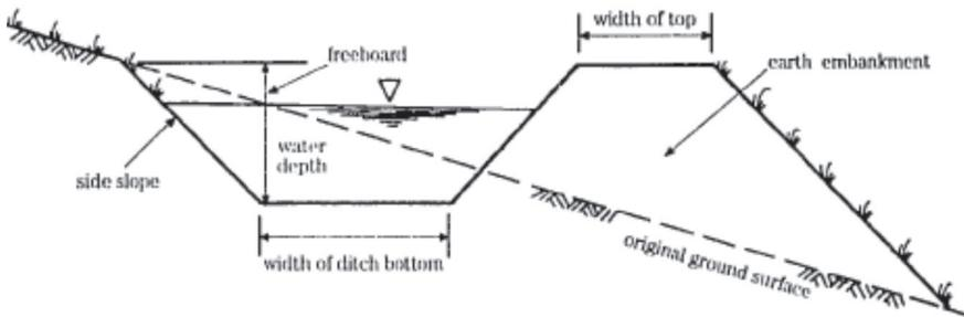
Figure 12-2: Cross section of a trapezoidal cut-off drain<sup>43</sup>
