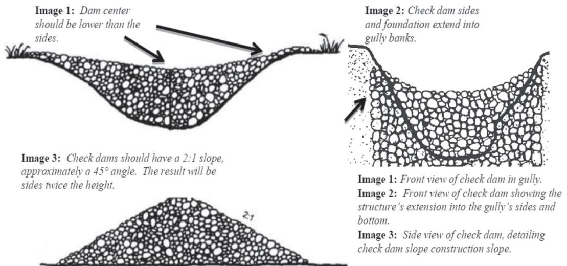
Figure 2-2: A stone check dam profile<sup>9</sup>
