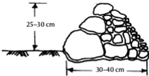
Figure 7-2: Cross section of a stone line<sup>27</sup>
