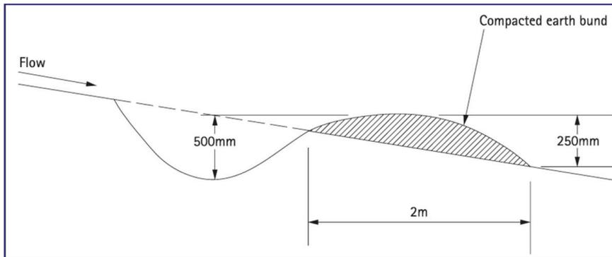
Figure 3-2: Cross section of a contour bund<sup>14</sup>
