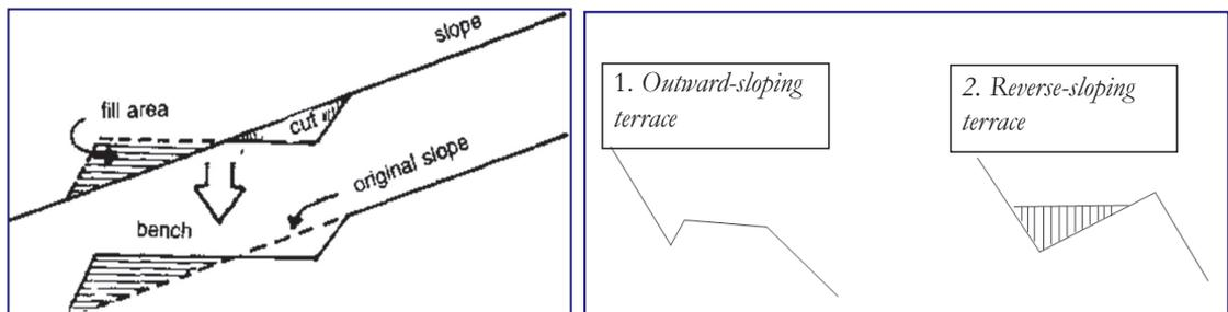
a) The cut and fill procedure used to construct bench terraces (b) Types of bench terraces in cross section
