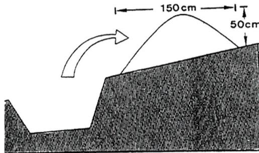
Figure 4-2: Construction of the *fanya juu* terrace<sup>20</sup>
