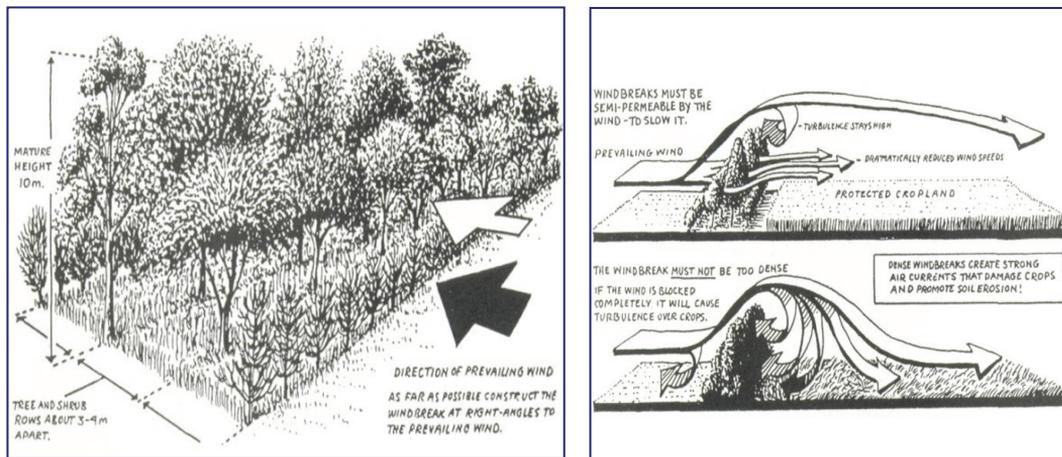
Figure 16-2: a) An illustration of a multi-storey windbreak b) Windbreak design<sup>44</sup>
