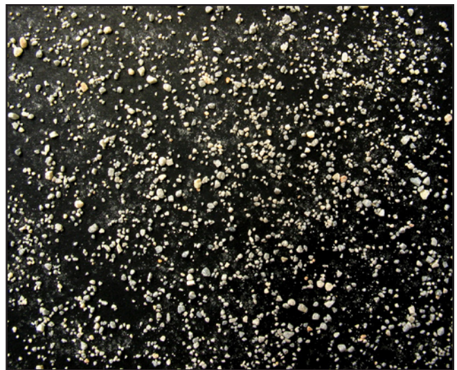
Fig. 3. Agricultural limestone particles ground to pass a 20-mesh sieve and retained on a 60-mesh sieve (i.e., -#20 +#60).
