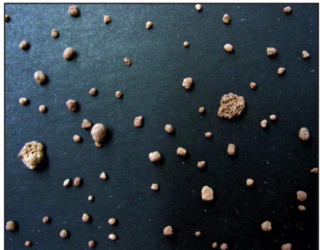
Fig. 7. Pelletized lime (#200 mesh ground limestone cemented into pellets that breakdown with soil moisture).
