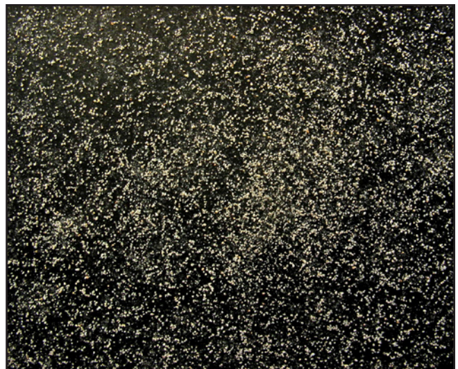
Fig. 4. Agricultural limestone particles ground to pass a 60-mesh sieve and retained on a 100-mesh sieve (i.e., -#60 +#100).
