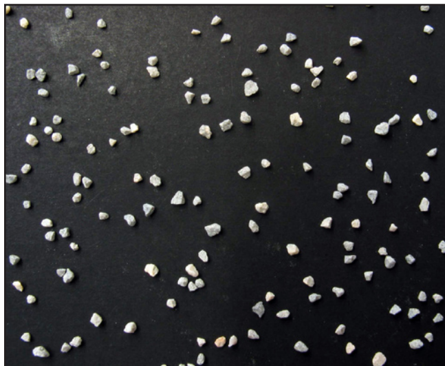
Fig. 2. Agricultural limestone particles ground to pass a 10-mesh sieve and retained on a 20-mesh sieve (i.e., -#10 +#20).
